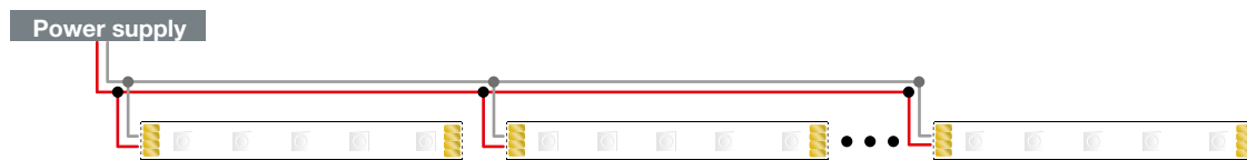
ELECTRICAL CONNECTION: connections in series or parallel
