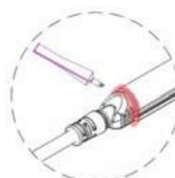
Add silicone glue in the groove for sealing
